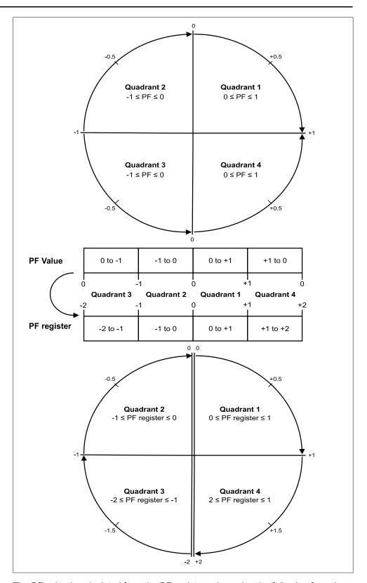
The PF value is calculated from the PF register value using the following formulae:
